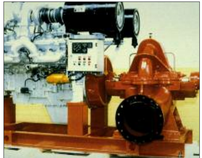
Pump sets. Coupling fitted between diesel engine and centrifugal pump.
