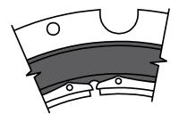
**Slotted rim (SLOT) -** A U-shaped cutout in the rim flange providing clearance for piping directly to the valve. Used with pipe adapter and in the small CB clutch applications which incorporate tapered bushings.
